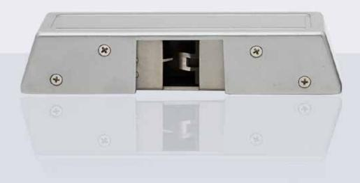
Lockwood Padde Series ES6000 Hook Lock is suitable for swinging doors, sliding doors and is easily attached to wood or steel door frames. ES6000 is heavy duty designed with its high preload (side load) capability of up to 300 kg, high holding force of up to 700 kg and up to 4hr fire rating. Both Power to Open and Power to Lock models are available.
