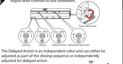
Closing sequence with Delayed Action 180° - 70° Control door speed with Delayed Action valve
