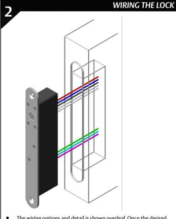
The wiring options and detail is shown overleaf. Once the desired wiring is chosen, run the wires into the rear of the mortice, and connect to the lock. There are screw terminals for each wire, and a connector guide is shown on the lock cover.
