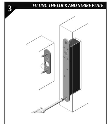
Slide the lock back into the mortice, making sure the wiring integrity is maintained. Secure the lock and strike plate in place, using the supplied mounting screws. Ensure that the hole behind the strike plate is free from swarf and is deep enough to allow the lock pin to fully extend when locked.
