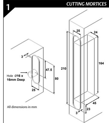
Cut mortices into the door and frame, for the strike plate and lock as per the dimensions shown. The top end of the strike plate must be aligned with the top of the lock, so the bolt pin goes centrally into the hole in the strike plate.
