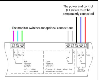
In either fail safe or fail secure configuration, maintained connection of '1' to '2' will keep the TB25 unlocked regardless of door position.
