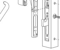
Assemble cylinder and secure with retainer pin. Ensure retainer pin is fully inserted to firmly anchor cylinder. Secure lever handle and opposing trim plate with 2 M4 X 65mm C'sunk head screws provided.
