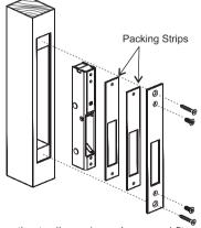
Cut mortice to dimensions shown and fit strike with 2 woodscrews supplied. If lock doesn't latch when door is closed, remove one or two packing strips.
