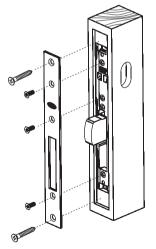
Secure Coverplate to lock with 3 M4 x 11mm C'sunk head screws provided. Secure Mortice lock to timber by 2 wood screws supplied.
