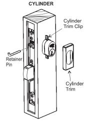
Assemble cylinder and secure with retainer pin . Ensure retainer pin is fully inserted to firmly anchor cylinder. Fit cylinder trim clip and cylinder trim.
