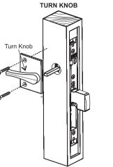
Cut connecting bar to allow 10mm to protrude from door face. Secure Turn Knob assembly with 2 small wood screws provided.
