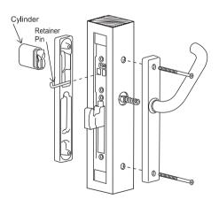
Assemble cylinder and secure with retainer pin. Ensure retainer pin is fully inserted to firmly anchor cylinder. Secure lever handle and opposing trim plate with 2 M4 X 65mm C'sunk head screws provided.
