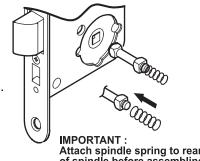
Attach spindle spring to rear of spindle before assembling
