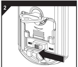
Slide the mode switch from the 'RUN' position to the 'SET' position. There will be a single beep and a red flash.
