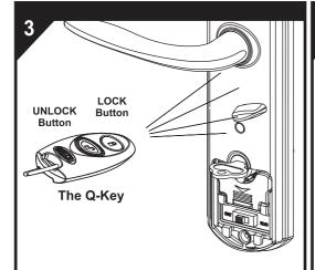
IMPORTANT: Once the first Q-Key is stored, all existing Q-Keys will be erased from the lockset's memory. All Q-Keys required to operate the lockset must be present when programming.
