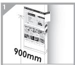
Mark line on the door face approximately 900mm from the floor. Tear along perforated line on template. Fold page along --- dashed line and place fold on door edge. Align CL with marked line on door face.
