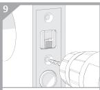
Insert bolt, then drill Ø2mm pilot hole and affix with screws provided.
