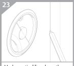
Mark a vertical line down the door jamb, along the edge of the
