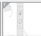
Insert bolt into Ø25mm hole, mark around latch face plate.
