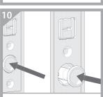
Press the retractable door pull button to release it. (Press to reset).
