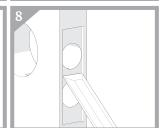
Chisel out recess to suit face plate. Face plate must be flush with door face.
