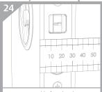
Measure and halve the door thickness.
