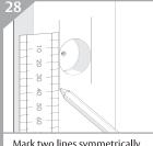
Mark two lines symmetrically either side of the Ø25mm hole centre line.
