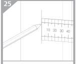
From the verical line on the door jamb, measure and mark half the door thickness. Draw a second line.
