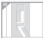
Chisel out strike plate recess. Strike plate must be flush with jamb.
