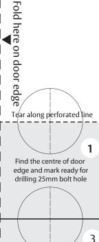
Find the centre of door edge and mark ready for drilling 25mm bolt hole
