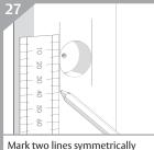
Mark two lines symmetrically either side of the Ø25mm hole centre line.
