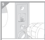
Insert bolt, then drill Ø2mm pilot holes and affix with screws provided.
