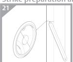
Partially close door and mark a horizontal line, centre of the latch bolt on the door jamb. Extend horizontal line along the inside face of the door jamb.
