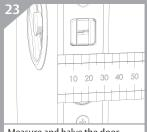
Measure and halve the door thickness.
