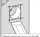
Chisel out basin recess to depth of hole.
