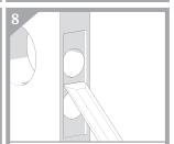
Chisel out recess to suit face plate. Face plate must be flush with door face.
